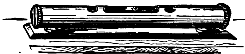
FIG. 45. A level somewhat like the levels used by carpenters. When the little air-bubble is in the middle of its tube, the straight-edged board is level—is horizontal.
